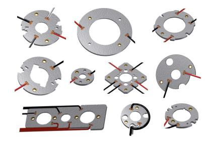
The holder improves the heat transfer from the COB to the heat sink and thermally disconnects the optics. Because of the mechanical integrity of micanite, the COB actually operates at a lower temperature which helps prevent premature LED failure.
